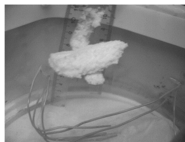
Figure 2: An ice crust which was removed from the top of a several cm thick ice sample, warmed by 1.1 solar constants for 1.5 h. Note the rugged ice structure [3].
