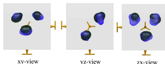
Figure 1: A comparison between exact (light blue) and recovered (dark green) anomalies recovered based on travel time data corresponding to three sources (yellow antenna symbols).
