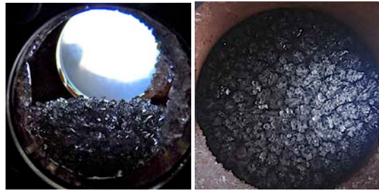
Figure 4: coarse grained CO 2 frost formation under a non-condensable atmosphere
