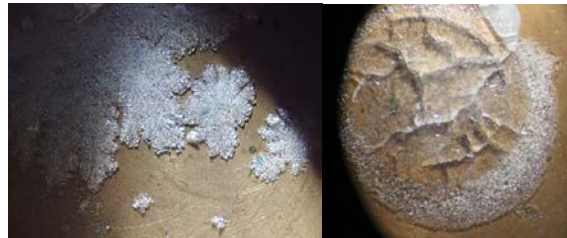
Figure 5: effects of positive (left) and negative (right) thermal stresses on a CO 2 slab.
