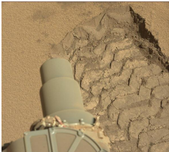
Fig. 4: MSL Curiosity, sol 530, rover wheel footprint presenting the behaviour of the sediment under pressure
