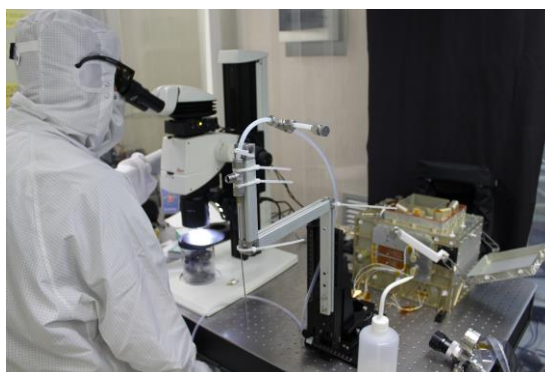
Figure 1: Set-up used for GIADA calibration using the cometary dust analogues.
