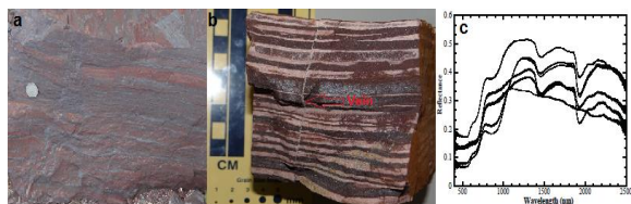
Figure 1: (a) Field photo depicting the Banded Iron Formation. (b) BIF with fault structure through which quartz vein is observed. (c) Reflectance spectra of hematite and goethite samples with characteristic absorption bands.
