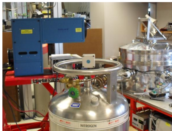
Figure 1: Laboratory set-up: Solar simulator (left), vacuum chamber (right), LN 2 dewar (front).
