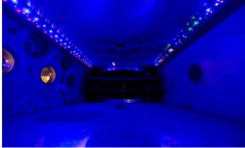
Figure 3 wind tunnel test section showing LED based illumination system (solar simulator).
