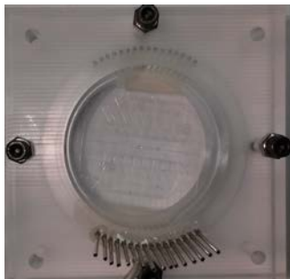
Figure 2: Rigid mount holding a 10+ year old automated \mu CE-LIF microdevice.
