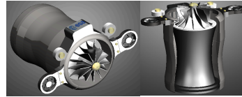
Figure 3: The design of the robot. It will be equipped with two cameras, 5 lamps, a big turbine in the center for fast movement, and two smaller rotators that can move in 45^\circ each side for sideways movement.
