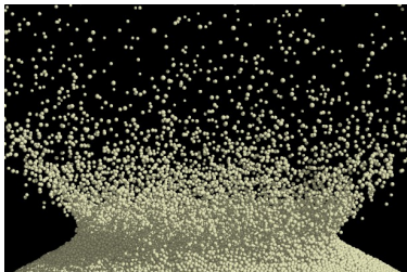
Figure 3: Ejecta grains after a simulated hypervelocity impact on a sandpile, running in space with intermittent collisions between.
