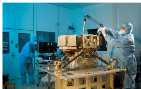
Figure 1: The JWST MIRI instrument in the RAL facility (UK) in 2012. The instrument features two main modules: an integral field spectrometer (on top) and an imager (at the bottom). For information about MIRI see [7]. (Copyright: Stephen Kill, STFC)
