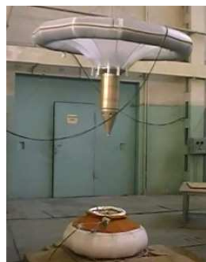
Figure 2: MetNet QM Penetrator and inflatable heat shielding.
