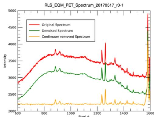
Figure 3: RLS EQM 1D spectrum of the PET calibration target. 1s Integration Time
