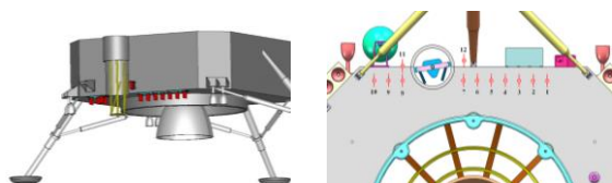
Figure 1: The lander model ground test setup. The LRPR is installed by one edge of the lander model's bottom, consisting of 12 separate antennas.
