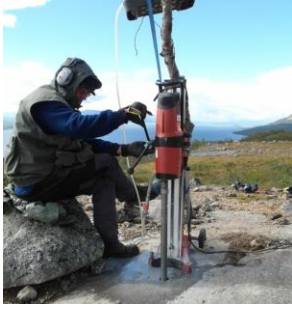
Figure 1. Drilling of Vakk-CH2B with a HILTI DD-200 (52mm drill crown)
