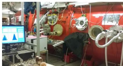
Figure 1 The main Planetary Simulation Facility under testing of the new liquid nitrogen atmospheric cooling system.
