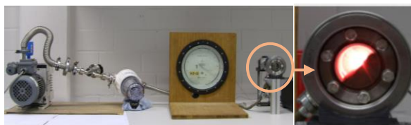
Figure 1: Rotating drum setup for dynamic angle of repose measurements
