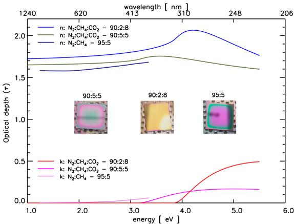
Figure 1: Refractive indices modeled for tholins prepared with different mixtures of  $N_2:CH_4:CO_2$ .
