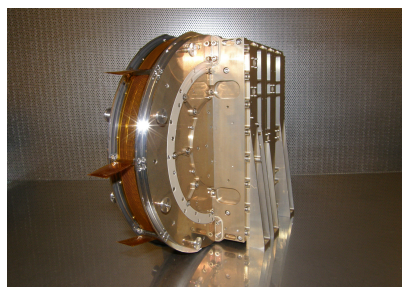
Figure 1: The flight model of the ENA instrument for BepiColombo, image credit: IRF
