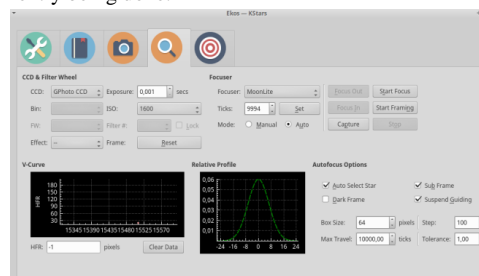
Figure 2 Interface for remote control of the telescope focus.
