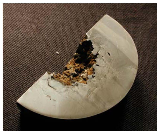
Figure 1: Sector of the ball from the Chinga meteorite after shock wave loading (diameter 56.01 mm).
