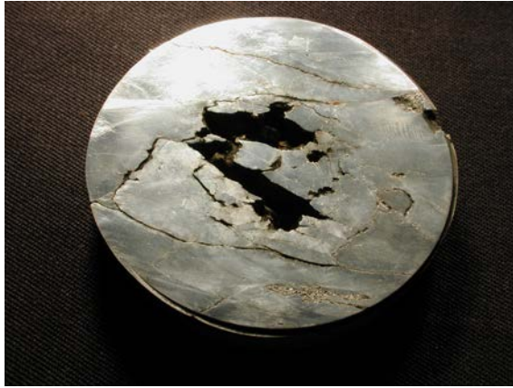
Figure 2: Cross-section of a ball from the Sikhote-Alin meteorite after shock wave loading (diameter 50.00 mm).
