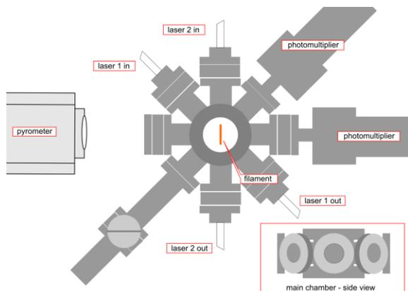
Figure 1: Top view of the MASI
