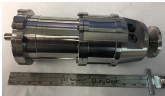
Figure 3: Vacuum micro-vessel with sapphire and diamond windows. Each window has a 5° field-of-view.
