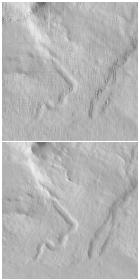
Figure 2: Results obtained using ASP only (top) and the proposed method (bottom). These shaded image sare produced when the sun azimuth is 256.63^\circ and the sun elevation is 50.20^\circ , same as for the left component of the CTX image pair.
