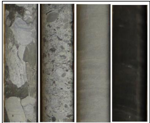
Figure 4. Representative lithological views of progressively fining upward core segments, 7.5 cm in length, from crater moat FC drill cores. From right to left: lower coarse breccia; finer upper breccia; fine upper breccia with clast size under the 5 mm cut-off grain size; and post-impact Chattanooga Shale.
