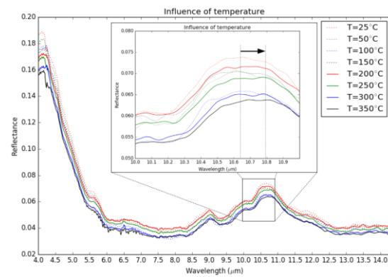
Fig. 1. Mid infrared spectra of a pellet of plagioclase taken at different temperatures (from 298 K to 623 K).
