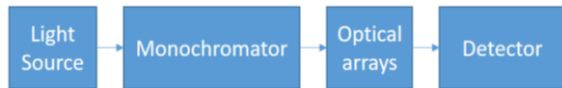
Figure 1: Preliminary schematic of the calibration bench. Optical arrays include the necessary elements to develop every measurement according to the configurations established: shutter closed, integrating sphere, and integrating sphere + focusing array, respectively. Some of these elements shall be inside of the vacuum chamber.
