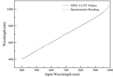
Figure 2: Graph to show offset of LVF wavelength
