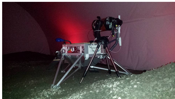
Fig. 4. ExoGeoLab lander from ILEWG equipped with VIS/IR spectrometer and telescope ready for use during EVA operations ( up ). Telerobotic operations using Modernity Rover ( down ).
