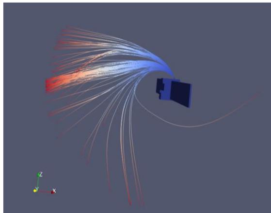
Figure 3: Simulation result from SPIS where low-energy  $\text{H}_2\text{O}^+$  ions are traced backwards from one of the sectors of the instrument. At the edge of the simulation volume these ions have an energy of approximately 2 eV. For further details about the simulation, see Figure 1.
