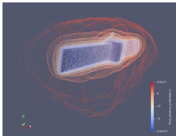
Figure 1: Simulated potential surfaces around the spacecraft. The spacecraft potential was for this simulation set to a fixed value of -20 V, the ion ( $\text{H}_2\text{O}^+$ ) and electron densities were set to  $1000 \text{ cm}^{-3}$ , and the ion and electron temperatures were set to 0.5 and 10 eV respectively. The drift velocity of the ions was set to 4 km/s in the  $-z$  direction.
