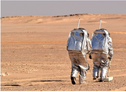
Figure 2: The analog astronauts during ScanMars experiment data acquisition. The radar sledge is being pulled along the planned profile.
