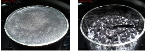
Figure 1: Change of the surface structure after 18 hours of irradiation. Sample includes 0.5% carbon black. T_0=173\text{K} , h_0 = 15\text{cm} .
