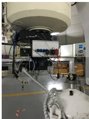
Figure 1: View of the Spectrograph mounted on the OGS telescope, showing the liquid N cooling system.
