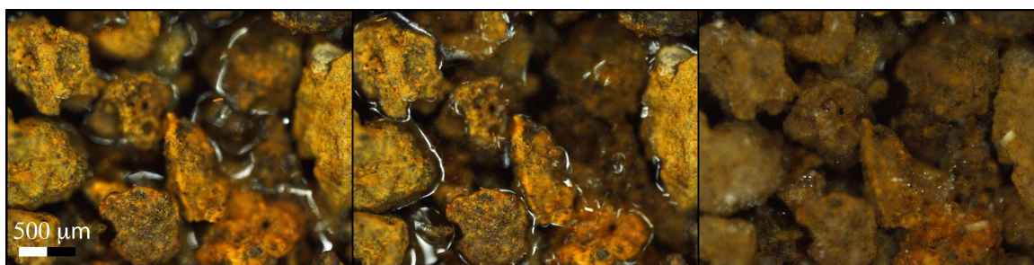
Figure 1: Sequence of microscopic images taken while CO 2 ice deposits in a form of slab ice under Martian conditions. From the left to middle frames CO 2 fills in the voids between the regolith particles. The right frame shows regolith completely covered by the ice.
