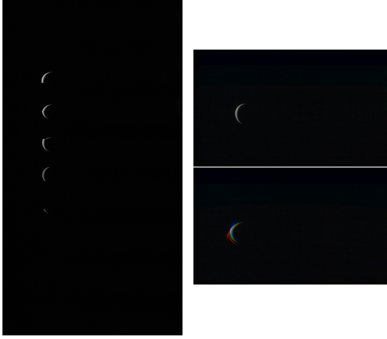
Figure 1: PJ12 approach image JNCE_2018090_12C00001_V01 with the raw in the left column, and two renditions in the right column, the upper rendition with well-chosen camera parameters, the lower one with a less appropriate Brownian K1 parameter.
