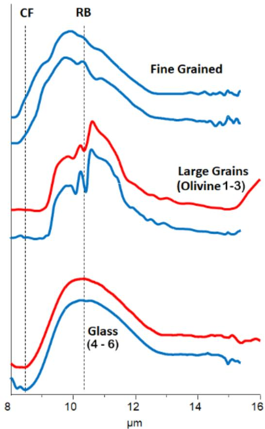
Fig. 2: Resulting micro-FTIR spectra from the pristine and melted parts of the basalt slab. Red = single point analyses (25 × 25 μm), blue = phases identified using PCS analyses.
