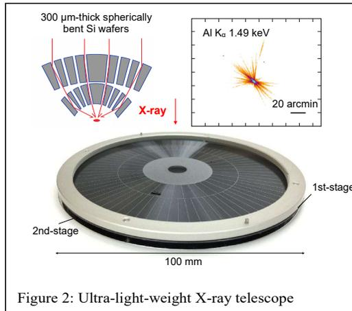
Figure 2: Ultra-light-weight X-ray telescope
