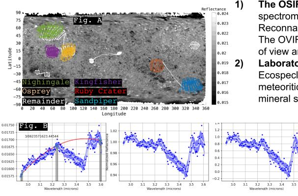
The OSIRIS-Rex data: data were collected from the OVIRS visible and infrared spectrometer and images were collected with the MapCam instrument in the Reconnaissance A mission phase from 09-September-2019 to 28-October-2019. The OVIRS observations are shown in Fig A. The size of the spectrometer Field's of view are roughly drawn to scale.
