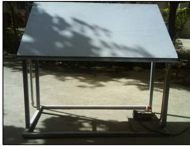
Figure 6: Proposed design for the water harvesting from air humidity system
