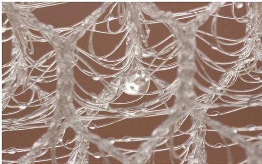
Fig. 1: Fibre-based fog collector with adhered water droplet
