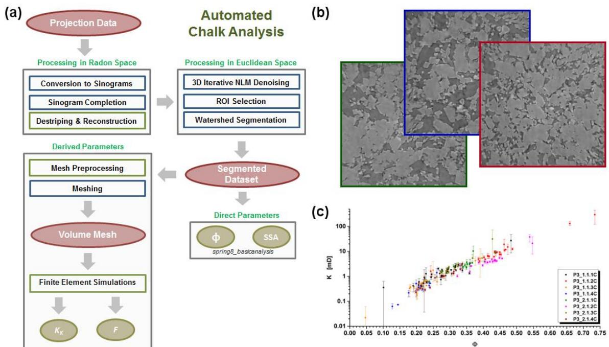
**Figure 1:** (a) Outline of the operations performed during the automated tomography image processing. (b) Examples of 2D slices after 3D iterative denoising and (c) the final results shown for the porosity-permeability.
