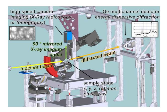
**Figure 1:** Overview of the instrumentation at the EDDI beamline, Bessy II, Berlin. The setup for simultaneous X-ray radioscopy/tomography with energy dispersive diffraction is composed mainly of a diffractometer and a high speed camera. The yellow line depicts the incident, the green one the transmitted and the orange one the diffracted beam. The insets shows a radiography of a liquid metallic foam (left) and the corresponding diffraction pattern (right).
