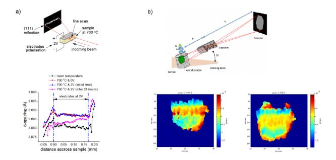
**Figure:** (a) top: setup of the local x-ray diffraction were the diffraction images are obtained from a line beam of 6 microns width and scans are performed in 50 positions across the sample. Bottom: gradient in lattice parameter observed between the electrodes after 24 hours under extreme operating conditions. In positive electrode (left side) the compressive stress is higher than in the negative electrode (right side), observable in the magenta line.
