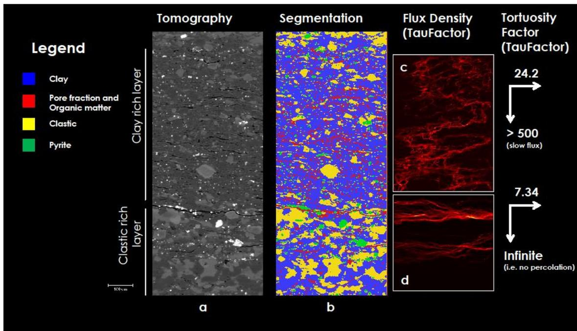
**Figure 1:** (a) Zeiss Xradia 520 Versa tomograph of a selected subvolume. (b) Segmented volume taking into account four main components of the shale rock: Clay, pores and organic matter, clastic phases (quartz, calcite and feldspar) and iron sulphide (pyrite). (c) Flux density map of the upper part of the sample. (d) Flux density map of the lower part of the investigated sample.
