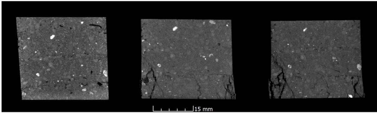
**Figure 1: CT images of the same fine-grained soil sample (similar to a clay), being progressively loaded (ex-situ) with cracks forming as the load increases. First failure occurred at 1.5 kN in this case shown in the middle image. Further loading increases the cracking as shown to the right.**
