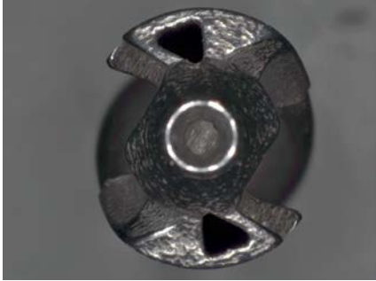
Figure 1: Tip of an additively manufactured cutting insert; ZEISS Smartzoom 5, 20×, ringlight, HDR
