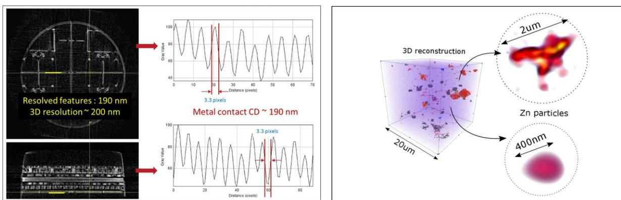
**Figure 1:** (left) analysis of metal lines in a semiconductor integrated circuit. Total acquisition time  $\sim 4.5$  hrs, 200 nm metal contacts are detected; (right) analysis of Zn particles and voids in Aluminum matrix. Total acquisition time  $\sim 6$  hrs, Zn particles down to 400 nm are detected.
