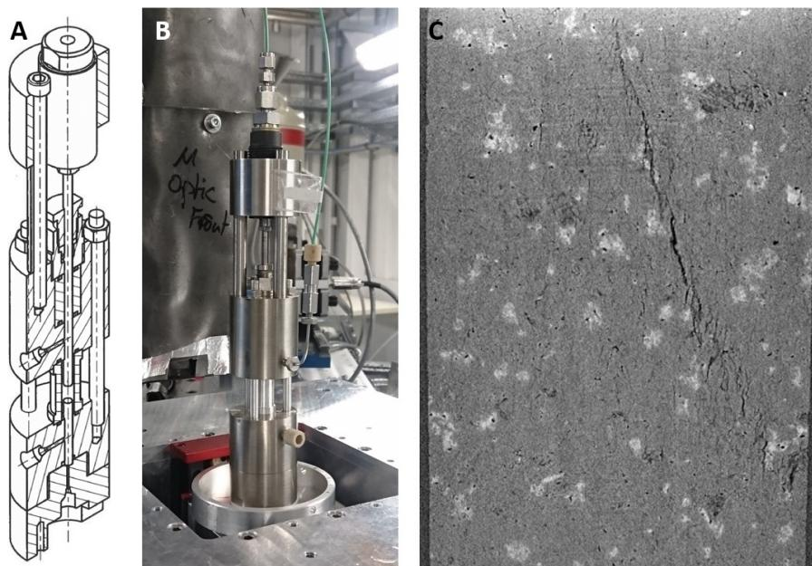
**Figure 1:** (a) Mjölnir in section and (b) in operation at the Psiché beamline on Soleil. (c) Shear failure in heat treated Ailsa Craig microgranite (FOV width ~3mm).
