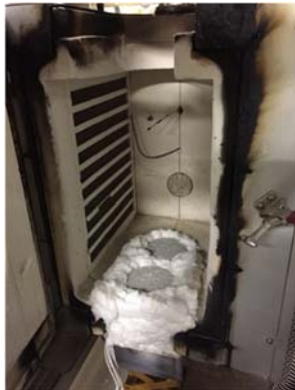
Figure 1: Situation of heating an end face of the specimen
